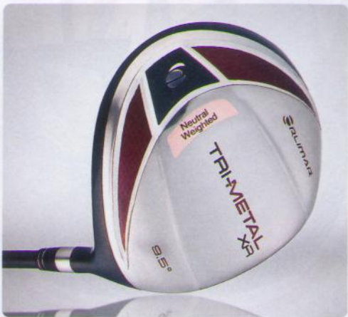
ORLIMAR TRIMETAL XR $180 The 6-4 titanium head uses a rear sole weight made of copper (twice the density of titanium) to lower the center of gravity.
